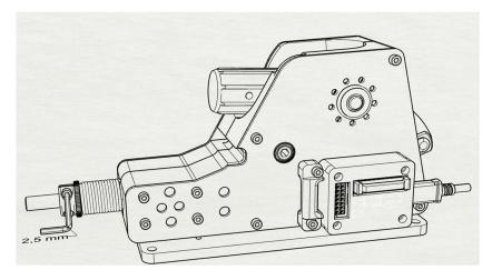
The upper position is reached by moving the inner ring. To do this, loosen one of the ring screws and leave the Allen key in the screw so that the ring stays in that position. Move the mechanism to the desired angle and fix the ring again.
