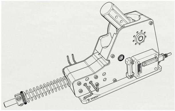
The holding force can be adjusted to your preference. A realistic setting would have to push the stick slightly upwards in the lowest position (spring fully tensioned).
